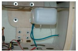
The fuel tank is included in the package, use cable ties or Velcro to secure in place
