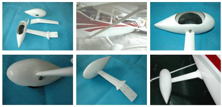
Install your wheel pants before you fit the legs to plane, cut slots the same as picture above make sure you fit the cuffs on the legs before you fit wheel pants on .Bolt landing gear on with the supplied Allen key bolts
