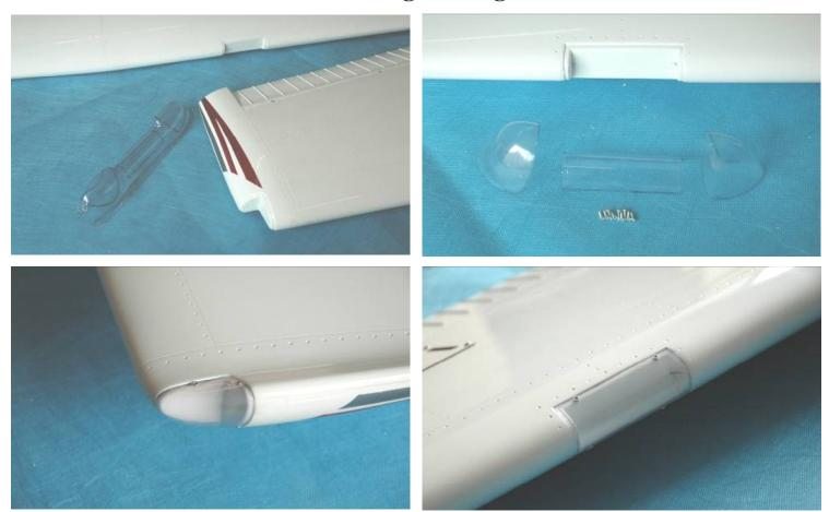
Cut the cover along the contour and use the 1.5mm screws supplied to secure in place
