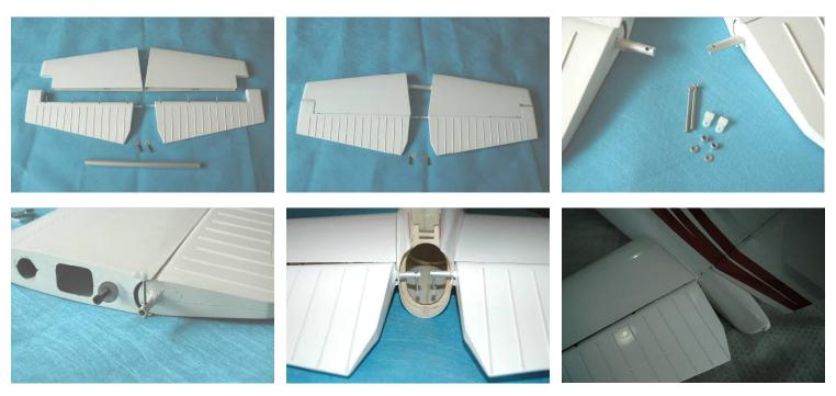
Insert the aluminum stab tube (22mm diameter) into the elevator, use 5\*25mm screws into the fixed elevator Install the push rod and check if it can be moved up and down properly.
