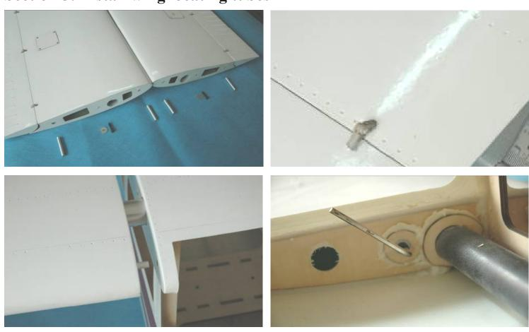
The package includes 4 aluminum locating tubes 8mm diameter Glue the small tube and leave 20mm distance
