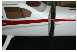
Using 4x5\*25mm screws to properly lock front and rear fuselage. MAKE SURE THESE ARE SECURE BEFORE FLYING
